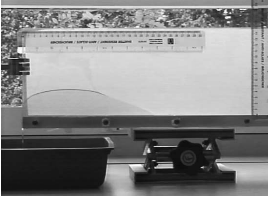
FIGURE 3. Photograph showing the experimental apparatus and the current slumping along the base of the Hele-Shaw cell.
